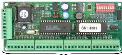
Clamp block for connection of pointing out contacts
